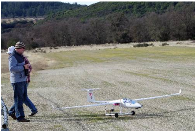
Tom's sailplane takeoff dolly. Large sailplanes can be a handful to launch and benefit from the takeoff dolly. Photo by Drew.
