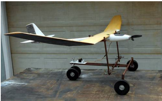
Doug's takeoff dolly for a sailplane. Doug's design is of welded steel square stock with a steerable tail wheel. Photo by Skjerseth.
