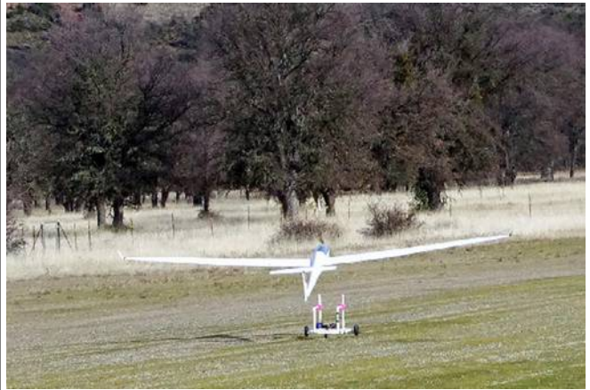
Takeoff dolly in action. Simple lightweight construction of PVC pipe and R/C wheels. Photo by Drew.
