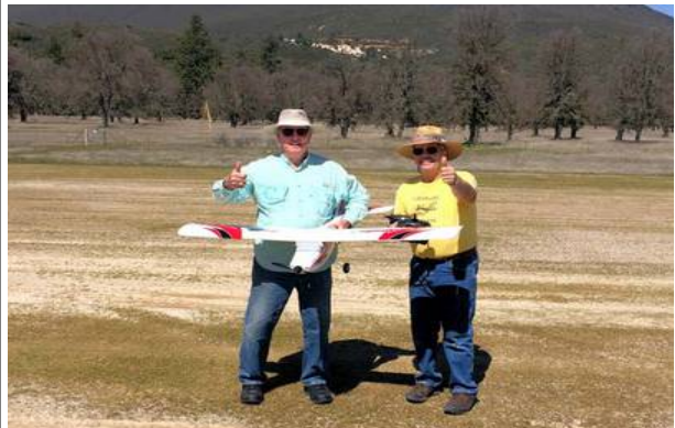
Jim Hiss and Scott Drew after a successful first flight. Jim is flying his Apprentice trainer which came equipped with two transmitter and a Bluetooth enable buddy box system. There are no wires between the two transmitters. (Dennis Locke photo)
